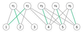
The Hopcroft-Karp algorithm [Hopcroft and Karp, 1973] allows for calculating the maximal matching in a bipartite graph
